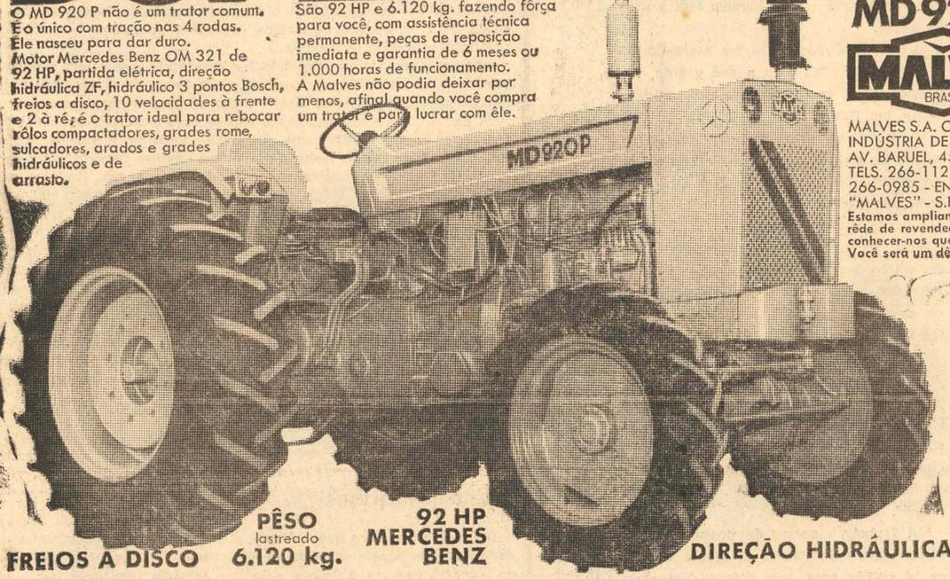
**FREIOS A DISCO** **PÊSO lastreado 6.120 kg.** **92 HP MERCEDES BENZ** **DIREÇÃO HIDRÁULICA**
