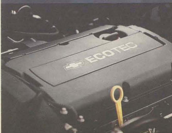
Novo motor Ecotec 6 1.8 Flex com dual CVVT.
